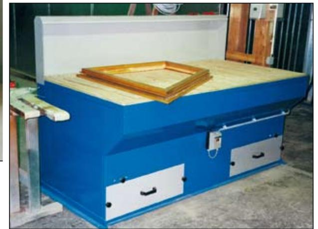
Sanding table is with built-in suction for sanding of all imaginable parts.
