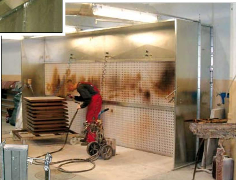
Automatic energy saving damper is controlled by a spray gun holder, opening when the operator uses the gun. This enables considerable energy savings.
