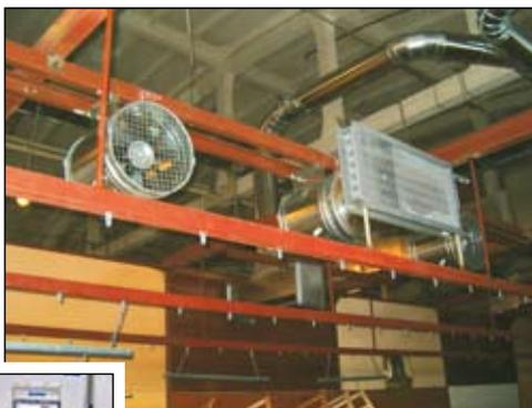
The drying process in our drying ovens is very economic and efficient, as the drying is effected with recirculated air.
