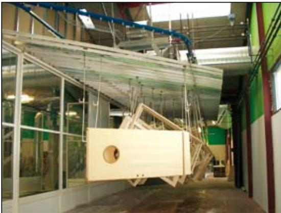
Suspension bar is hung up on two parallel conveyor paths guarantying stable operation, though heavy elements are transported.
