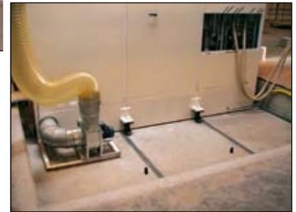
A solution with 2 flowcoaters for quick change of colour/liquid is shown here. Flowcoater is on running rails and is displaced sideways in proportion to the parts.
