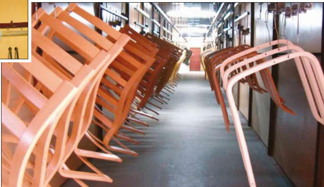
Conveyor system for transport of special plastic parts through the drying process.
